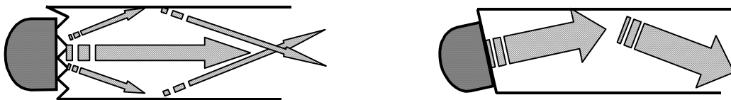
Figure 2 Rough and angled transducer contact
