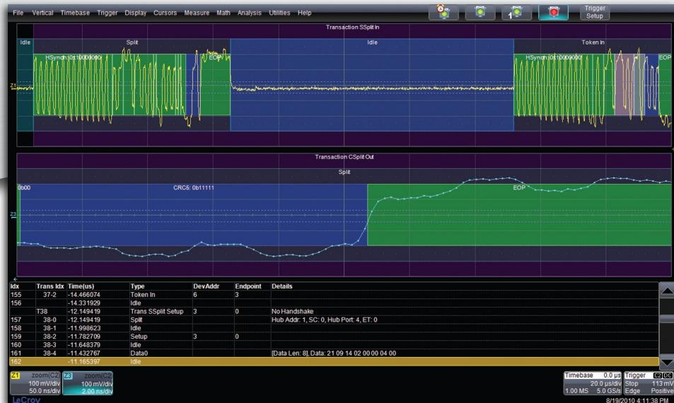
The comprehensive triggering, intuitive decode and easy to navigate table display enable a powerful tool set to quickly debug a USB device or system.
