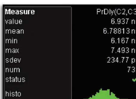
Quickly measure channel properties with measurement parameters defined by the FlexRay specification. Teledyne LeCroy's statistical measurements with histograms, tracks and trends let you see how the channel behaves over time.
