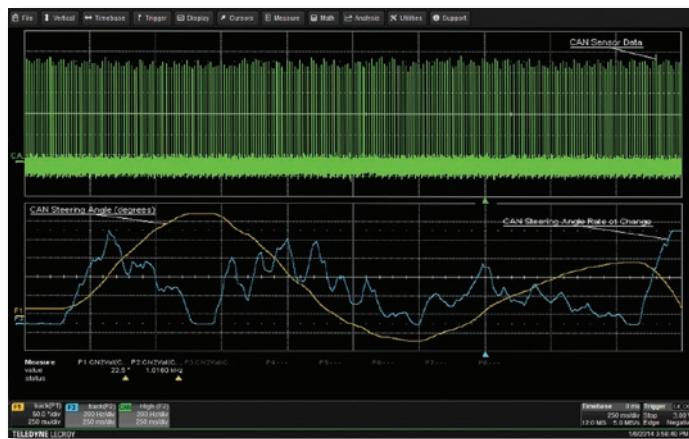
Here, information on the steering angle and steering angle rate of change is extracted from the CAN message acquisition, rescaled to decimal values, and plotted as a time-correlated "Track"
