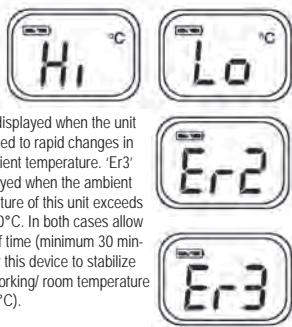
'Er2' is displayed when the unit is exposed to rapid changes in the ambient temperature. 'Er3' is displayed when the ambient temperature of this unit exceeds -10 to 50°C. In both cases allow plenty of time (minimum 30 minutes) for this device to stabilize to the working/ room temperature (0 to 40°C).
