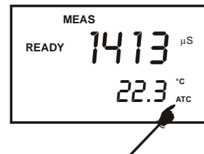
Figure 15: Automatic Temperature Compensation
