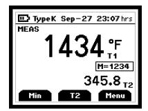
On initial start-up the meter will display the measured value for input one in the primary display and for input two in the secondary display.
