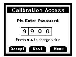
Before go into the calibration mode, must enter the password. Press F2 to change to the next digit. (Default Password is 9900)
