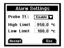
Disable or enable the alarm for individual probe by pressing recall ▲ or log ▼ and F1 to accept. Increase or decrease individual limit by pressing recall ▲ or log ▼.
