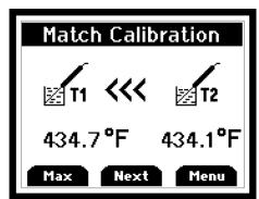
Use the ▲ or ▼ keys to adjust the value to match T1 readings and T2 readings.
