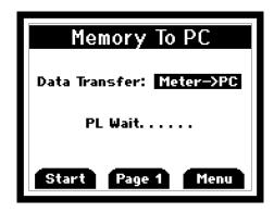
Once the USB connection is establish with PC, press the Start button to download data from Meter to PC using HyperTerminal.
