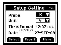
Press *F1* to indicate you want to change the setting of the current parameter or recall ▲ or log ▼ to move to the next parameter.
