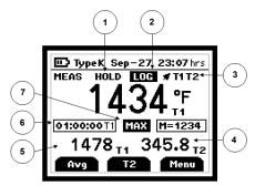
The dot matrix display features a large primary display, smaller secondary displays for channel info or min/max/ave, and helpful annuciators for added measurement data
