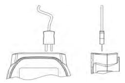
If no probe is connected the display will read "open".
