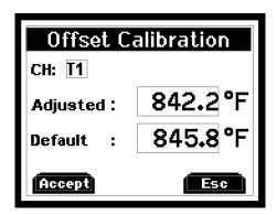
Use the ▲ or ▼ keys to adjust the value to match known temperature standard. Press *F1* to accept.
