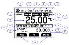
The dot matrix display features a large primary display, smaller secondary displays for channel info or min/max/ave, and helpful annuciators for added measurement data
