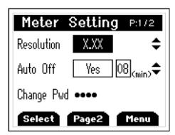
Press *F1* to indicate you want to change the setting of the current parameter or recall ▲ or log ▼ to move to the next parameter.
