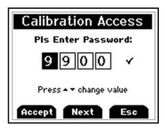
Before go into the calibration mode, must enter the password. Press F2 to change to the next digit. (Default Password is 9900)
