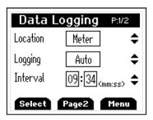
Press recall ▲ or log ▼to choose the logging methods as auto or manual. If it is auto logging, using recall ▲ or log ▼to set time interval. Its range is from 2min to 60min.
