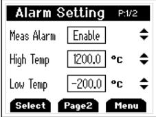
Disable or enable the alarm by pressing recall ▲ or log ▼ and F1 to accept. Increase or decrease individual limit by pressing recall ▲ or log ▼.
