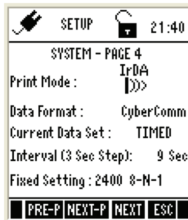
Figure 5: System Settings Page 4 – Wireless Serial Data Communication
