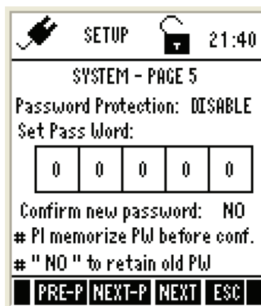
Figure 6: System Settings Page 5 – Password Protection
