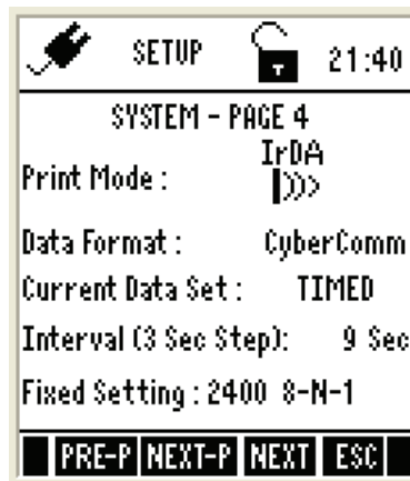
Figure 5: System Settings Page 4 – Wireless Serial Data Communication
