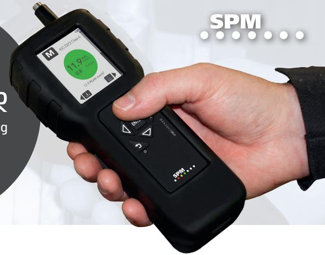
VibChecker is a compact-sized instrument for vibration measurement in the 10-1000 Hz frequency range. Measurement results are immediately and automatically evaluated against ISO standards with a clear, intuitive indication of vibration severity. Time signals and real-time FFT spectrums enable easy pattern recognition. Measurement results can be stored for trending of vibration levels and follow-up.
