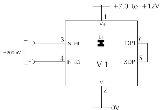
Measuring an input voltage referenced to a floating supply, i.e. the input voltage and the meter's power supply are isolated from each other. Check Link L1 is closed.
