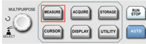
Figure 7-1 Function Key of Auto Measurement
