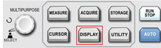
Figure 6-1 Function Keys of Display System
