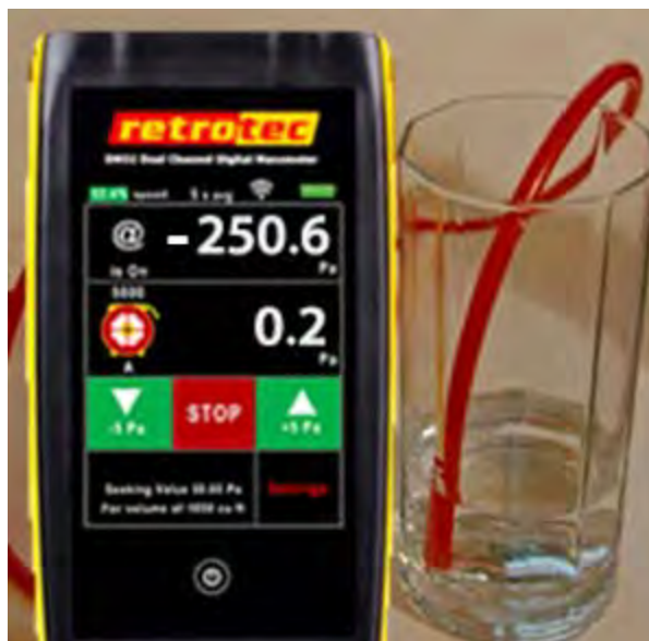
Figure 71: The gauge displaying a negative pressure (-250.6 Pa).
