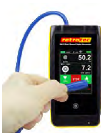
Figure 67: Errors in pressure reading from a pinched tube.
