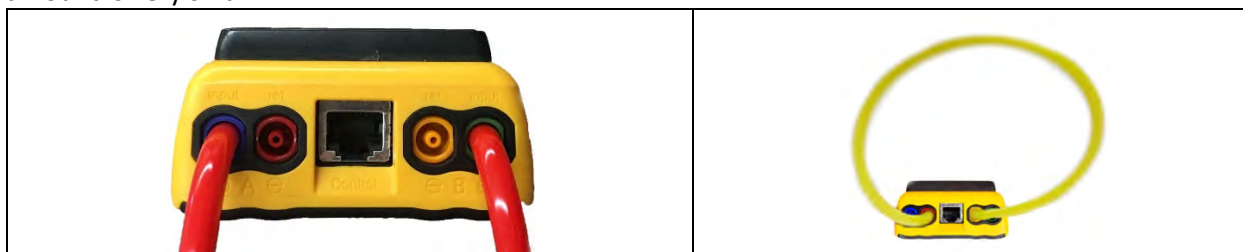
Figure 65: Gauge field check configuration: Cross port check, input ports (left) and reference ports (right)
