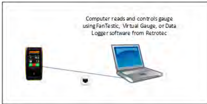
Figure 52: Use "Network" connector to connect a single gauge to a computer
