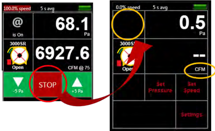
Figure 33: Stopping fan disables and turns [ @ Pressure ] off
