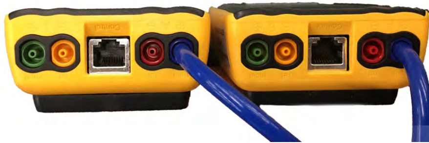
Figure 66: Gauge field check configuration: Cross gauge check
