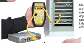
Go INLINE between two LAN devices and the TVR10/100/1000 will check the speed and duplex of the link (this is termed negotiated speed). The ability to test negotiated speed in this price range is unheard of! Plus, it detects PoE (Power over Ethernet). Both endspan and midspan.
