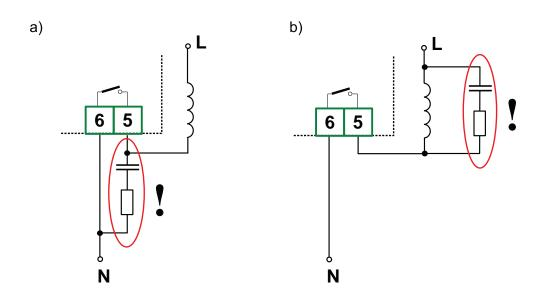
Figure: Examples of Suppression Circuit Connection
