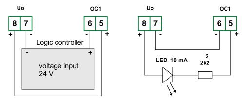
Figure: Examples of OC-type output connection
