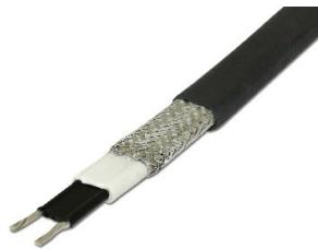
Increasingly used for underfloor and similar applications, but the most common use for this is thermal protection of pipelines from frost. Self-regulating cable is easy to simply wrap around and along the pipeline beneath any insulation. The surface of the tape will reach a known temperature without additional hardware (no thermostat required, but
