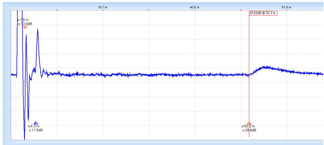
Now it is easy to identify where along the cable a break has occurred from the trace. In this case, I've simply removed the shorting link from the end of a two-core heating cable, so you can see the end-of-cable event has changed from a "short" to an "open" (above the line event). Similarly, should a "short" be found earlier along the cable than expected then you would suspect damage, perhaps by crushing at that point.
