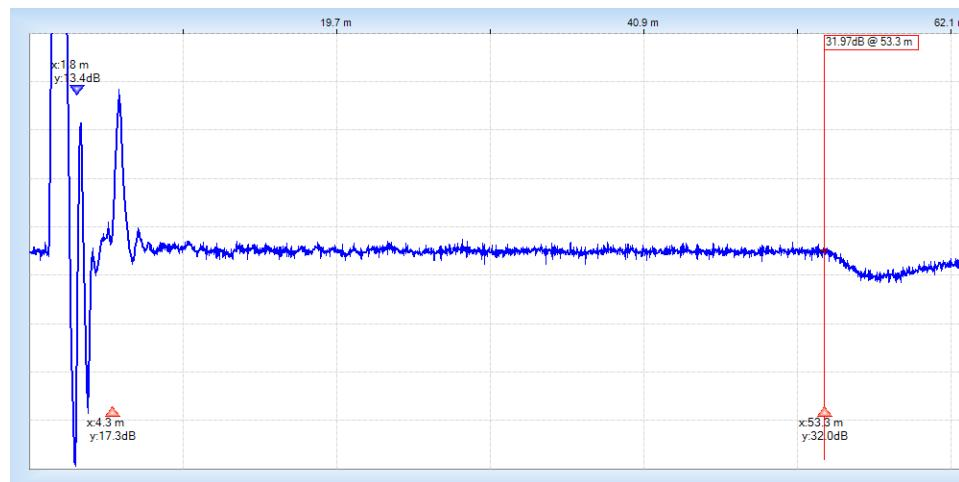
In this trace for example, the transition from the TDR's own patch cable to the “cold tail” is at 1.8m. The end of the “cold tail” where it joins the heating cable is the high impedance at 4.3m and the end of cable is at 53.3m; shown here as a “below the line” “short” event where the end of cable link is found. This is an example of a 4.0m<sup>2</sup> pre-made dual core plus screen “mat”.
