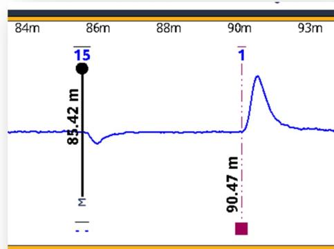
This screenshot from a Tempo TV220E TDR shows the transition from  $75\Omega$  to  $50\Omega$  and the open "end-of-cable". The event return loss figures are above each marker.
