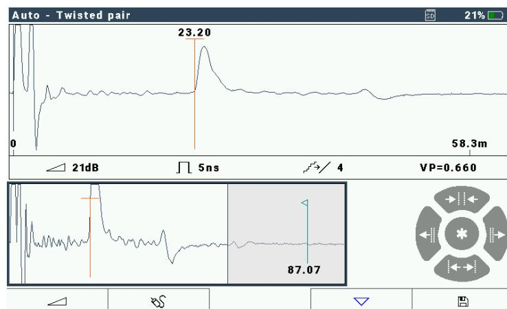
This cable is 23 m long and apart from the open end shows no significant trouble.
