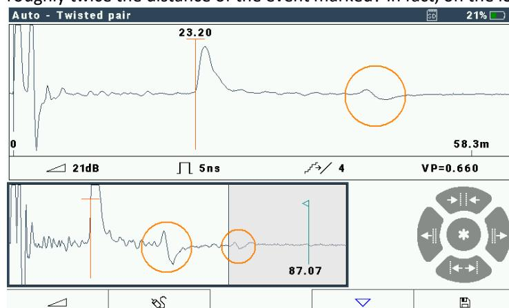
trace you can see two of them. They are “Ghost reflections” where the part of the energy from the original reflection meets the mismatch near the transmitter and goes around the loop again (and again, attenuated by about 17 dB plus the cable losses each time).
