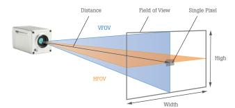
HFOV - Horizontal Field of View (horizontal aperture angle) VFOV - Vertical Field of View (vertical aperture angle)
