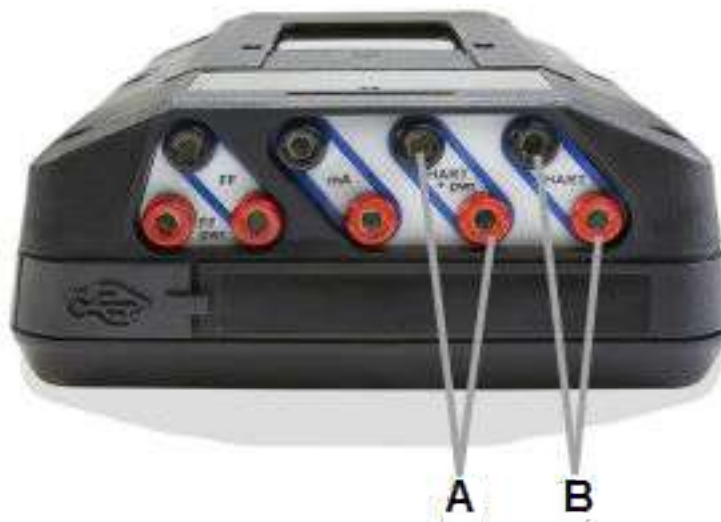
Figure 3-10: HART communication terminals on the Device Communicator Plus communication module
