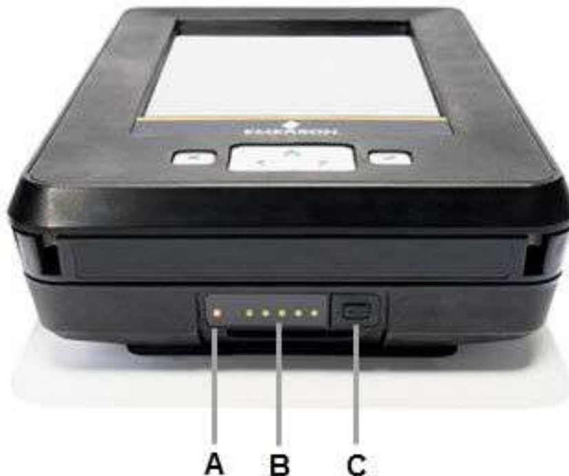
Figure 2-9: LEDs showing approximately 100 percent charge
