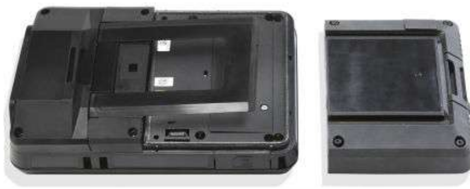
Figure 2-10: Trex unit with the power module removed
