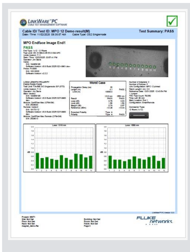
LinkWare PC report showing end face image and loss results (including PASS for each) for a 12-fiber MPO cable.
