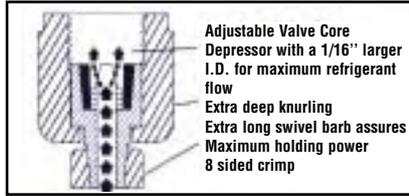
Adjustable Valve Core Depressor with a 1/16" larger I.D. for maximum refrigerant flow
