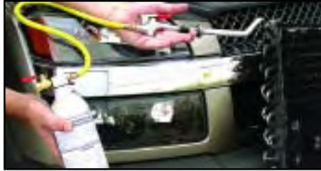
Reduce comebacks by flushing evaporator & condenser with the **TLFG**. Simply add solvent and use shop air to reverse flush the component. **TLFGXT** - Replacement tip for flush gun.
