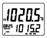
T2 present reading + T2 Maximum reading plus elapsed time + T2 Minimum reading plus elapsed time + T2 Averaging reading plus averaging time.
