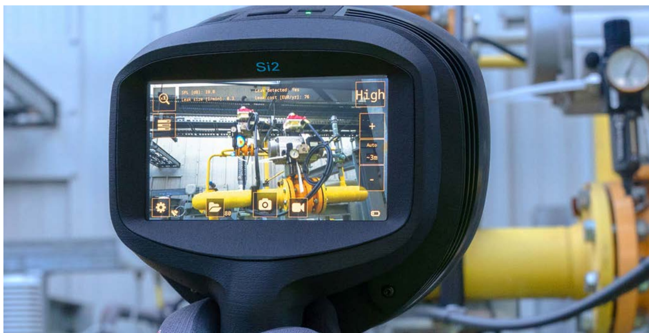
FLIR Si2 leak detection acoustic imager in the field calculating leak size and cost of leak.
