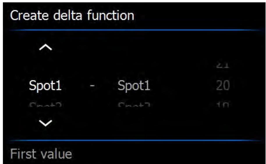
3. Push the joystick. The result of the difference calculation is now displayed on the screen.
