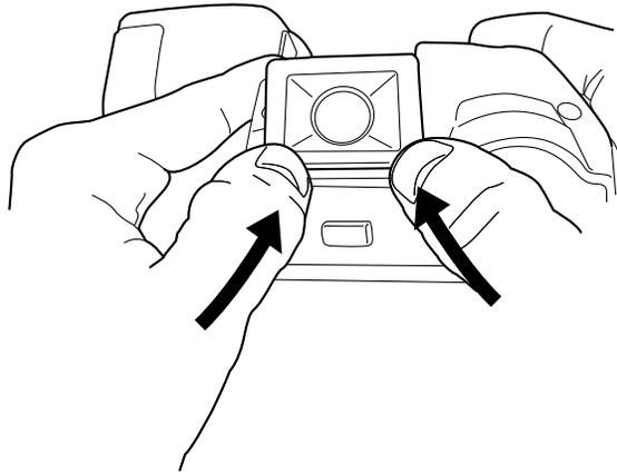
2. Note the grooves on the eyecup mount on the camera and on the new eyecup.
