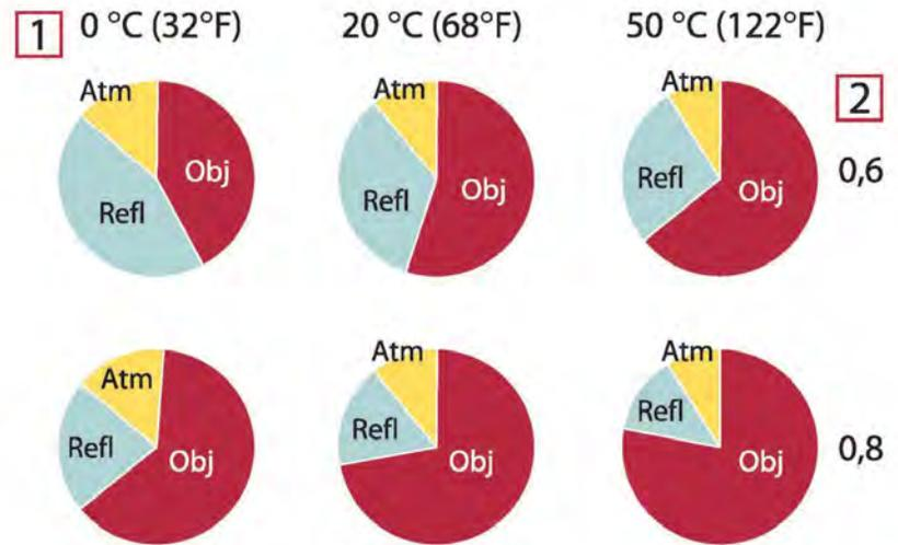
**Figure 34.3** Relative magnitudes of radiation sources under varying measurement conditions (LW camera). 1: Object temperature; 2: Emittance; Obj: Object radiation; Refl: Reflected radiation; Atm: atmosphere radiation. Fixed parameters:  $\tau = 0.88$ ;  $T_{refl} = 20^{\circ}\text{C}$  (+68°F);  $T_{atm} = 20^{\circ}\text{C}$  (+68°F).
