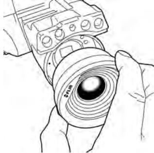
7. Carefully push the lens into position.
