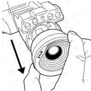
4. The infrared detector is now fully exposed. Do not touch this surface. If you see dust on the detector, follow the instructions in 27.3 *Infrared detector*, page 484.
