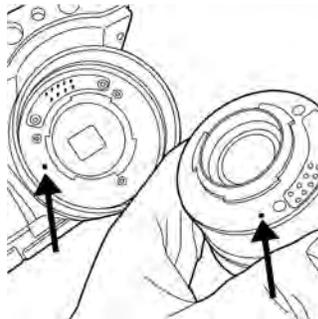
6. Align the lens correctly to the bayonet mount.
