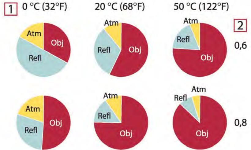
**Figure 34.2** Relative magnitudes of radiation sources under varying measurement conditions (SW camera). 1: Object temperature; 2: Emittance; Obj: Object radiation; Refl: Reflected radiation; Atm: atmosphere radiation. Fixed parameters:  $\tau = 0.88$ ;  $T_{refl} = 20^{\circ}\text{C}$  (+68°F);  $T_{atm} = 20^{\circ}\text{C}$  (+68°F).
