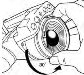
3. Carefully pull out the lens from the lens bayonet mount.
