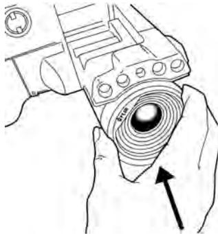
8. Rotate the lens 30° degrees clockwise.
