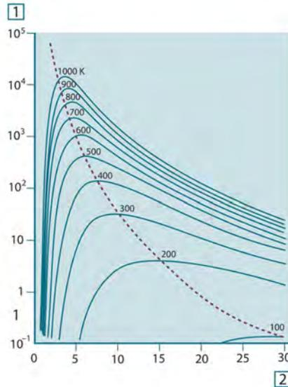
**Figure 33.6** Planckian curves plotted on semi-log scales from 100 K to 1000 K. The dotted line represents the locus of maximum radiant emittance at each temperature as described by Wien's displacement law. 1: Spectral radiant emittance ( $\text{W}/\text{cm}^2$  ( $\mu\text{m}$ )); 2: Wavelength ( $\mu\text{m}$ ).
