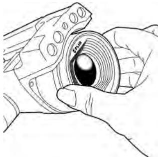
2. Rotate the lens 30° degrees counter-clockwise.
