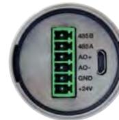
Thermalert 4.0 with 6-pin terminal providing analog out and RS-485 communications
