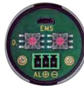
Thermalert 4.0 supports 2-wire loop for simultaneous power supply and analog output
