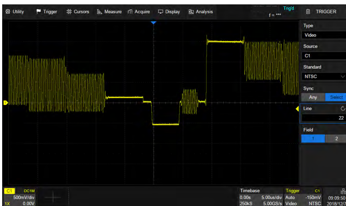
Trigger on a Specific Line of Video(NTSC)
