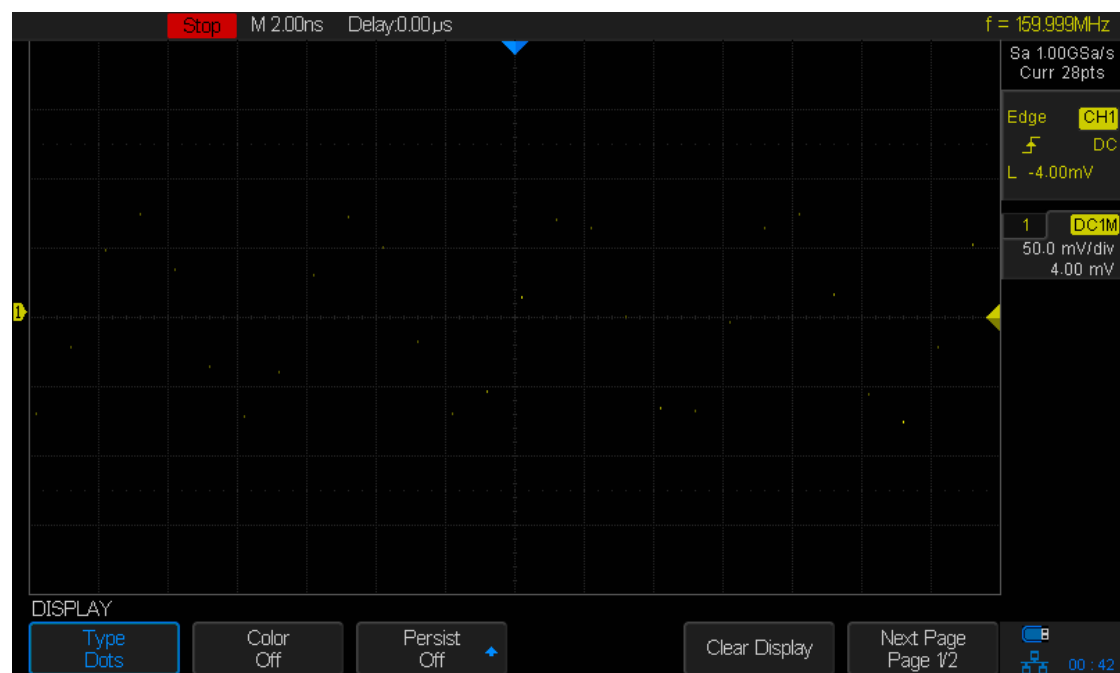
Figure 11: Display Type Set to Dots
