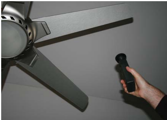
ST-1000 Checking Fan Speed and Balance
