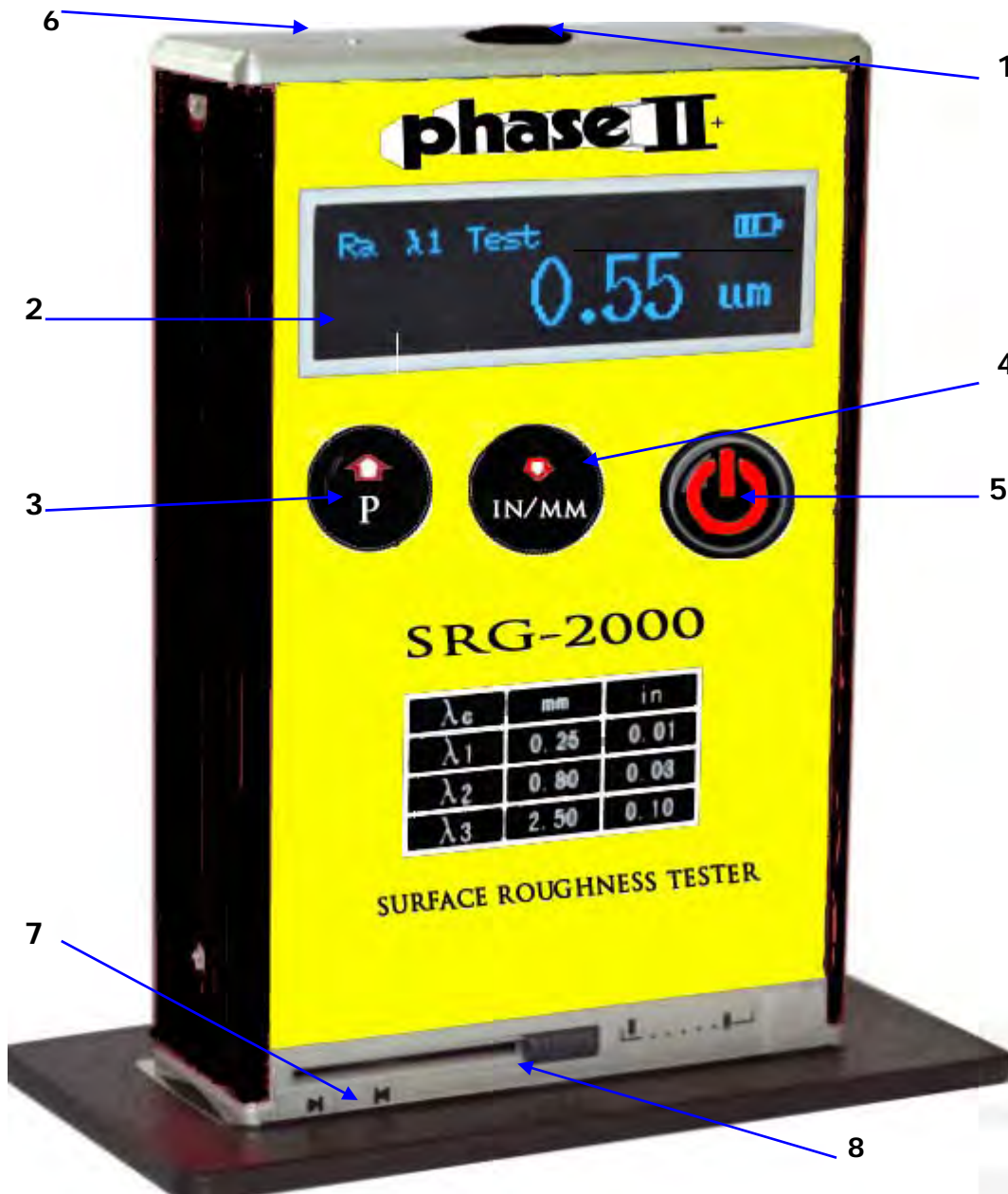
FIGURE 2: STRUCTURE OF MAINFRAME
