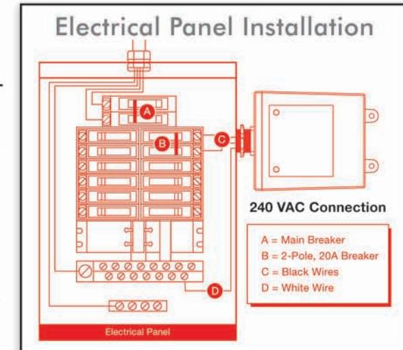
All conductor lengths should be as short as possible and bends should not be sharp; a 4" bend radius or wider is recommended. **DO NOT LOOP OR COIL WIRES.**
