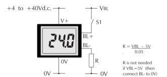
Powering the LED backlighting from a separate supply. Close switch S1 to turn on the backlighting.
