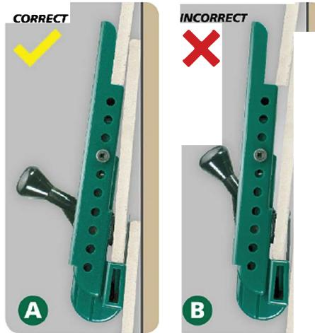
**NOTE:** Over-tightening handle may cause tool to pull away from siding. As the rubber pad naturally wears over time, the handle can be engaged further for continued use.
