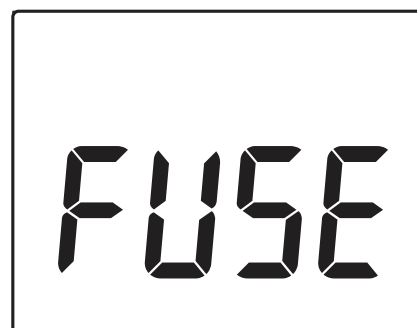
Fuse blown out
