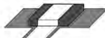
Figure 14A Current Sensing Resistor mounted on a Printed Circuit Board
