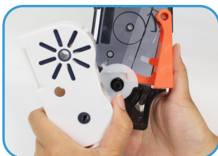
2. Remove side cover and cartridge
