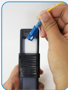
Wipe connector ferrule across cleaning surface
