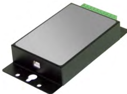
Figure 52: USB/RS485 Adapter (XXXUSB485)
