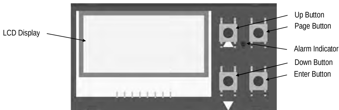
Figure 33: Control Panel for the Comm Box (DIN)
