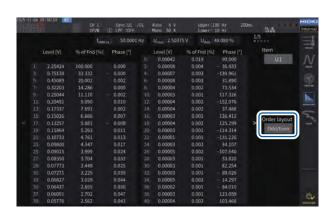
Select to display a list with odd-order measured values arranged on the left side of the screen and even-order measured values on the right side. Three types of measured values (RMS values, harmonic factors, and phase angles) of voltage, current, and power are displayed from the 0th to 40th orders on a single screen.
