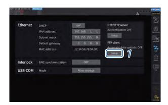
Tap the [Setup] box under [FTP client] to open the setting window.
