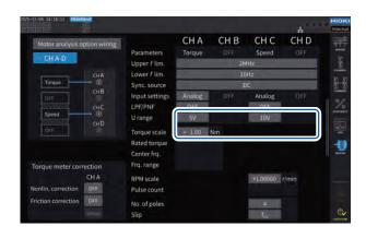
Example: For a torque sensor with a rated torque of 500 N·m and an output scale of ±10 V
