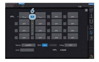
You can select the basic measurement parameters on the parameter selection window. (Other UDF calculation results can also be selected as parameters.)
