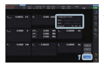
When the integration control is set to [All Channel], the [Integration Time] field displays the integration start time, integration stop time, and elapsed time common to all wiring configurations.
