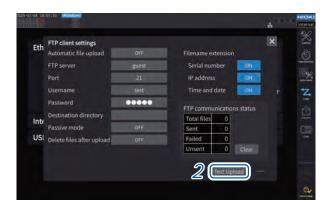
7 Tap the [Setup] box under [FTP client] to open the setting window.
