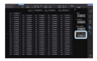
Select to display all orders side by side in one column. One type of measured values are displayed from the 0th to 50th or 100th orders on a single screen.
