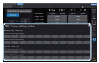
When the torque meter to be used provides calibration values, you can compensate for errors of the torque meter by entering the target values and calibration points.
