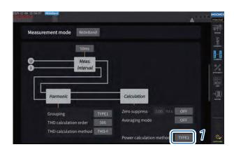
Tap the [Power calculation method] box, then select the calculation type from the list.
