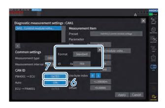
Tap the [Auto] box to select the automatic setting of the format and ID of the CAN signal returned as a response from the ECU.
