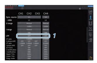
Tap the [LPF] box of the wiring configuration you wish to set and select a low-pass filter from the list.
