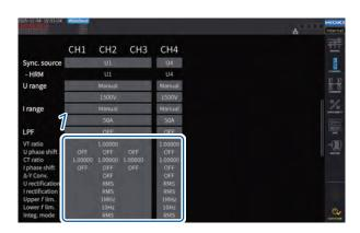
Tap the channel detail display area for the channel you wish to configure to open the settings window.
