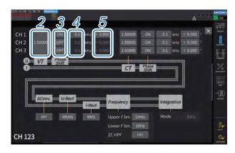
2 Tap the [VT] box and enter [1000.00] using the numeric keypad.
