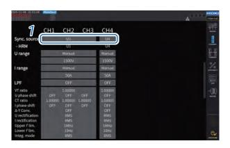
Tap the [Sync. source] box of the wiring configuration you wish to set to open the setting window.
