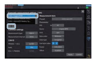
(To also acquire other CAN data) Tap [+] at the top left of the diagnostic measurement setting window to add a CAN setting.
