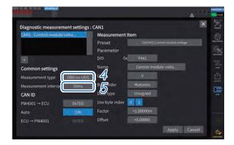
Tap the [Measurement type] box and select a measurement type.
