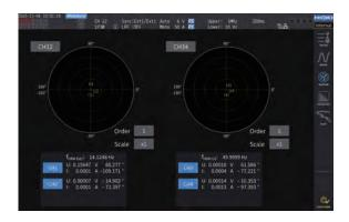
The 2-vector-diagram display illustrates two graphs of each selected wiring configuration.
