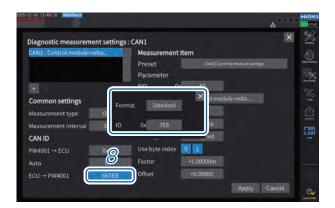
When [OFF] is selected for [Auto], tap the [ECU→PW4001] box to set the format and ID of the CAN signal returned as a response from the ECU.
