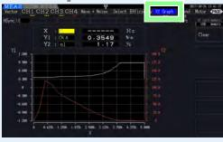
This page displays an X-Y graph of mea- This page displays fluctuations of up to surement parameters selected for hori- eight measured values. zontal and vertical axes.
