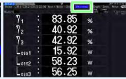
This page displays the numerical values of efficiency and loss determined by calculation formulas.
