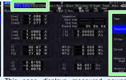
This page displays measured power, voltage and current values, integration values, and provides access to harmonic graphs and lists for each channel.
