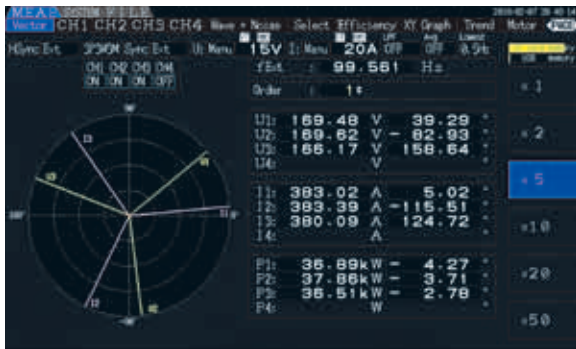
Display motor electric angles on the vector screen
