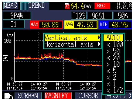
**3** Select the desired zoom factor with the cursor keys and press the
