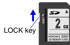
**4** Positioning the SD memory card with the top surface facing up, insert it into the slot in the direction shown by the arrow and push it all the way in.
