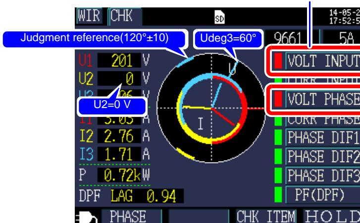
Udeg3 will be  $60^\circ$ , causing a voltage phase failure since it falls outside the judgment reference ( $120^\circ \pm 10^\circ$ ).
