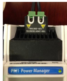
PM1 top view - 100~240VAC input terminals
