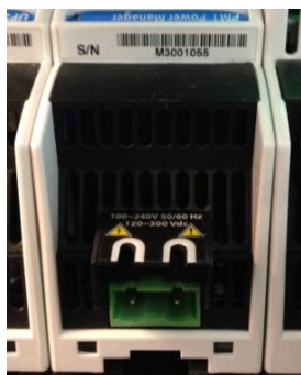
PM1/PM2 rear view - 100~240VAC input terminals
