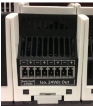
PM2 front view – 24VDC output terminals
