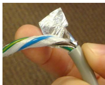
Figure 2: To minimize emissions with the optional PM1 Power Supply module, optionally use a shielded power conductor.
