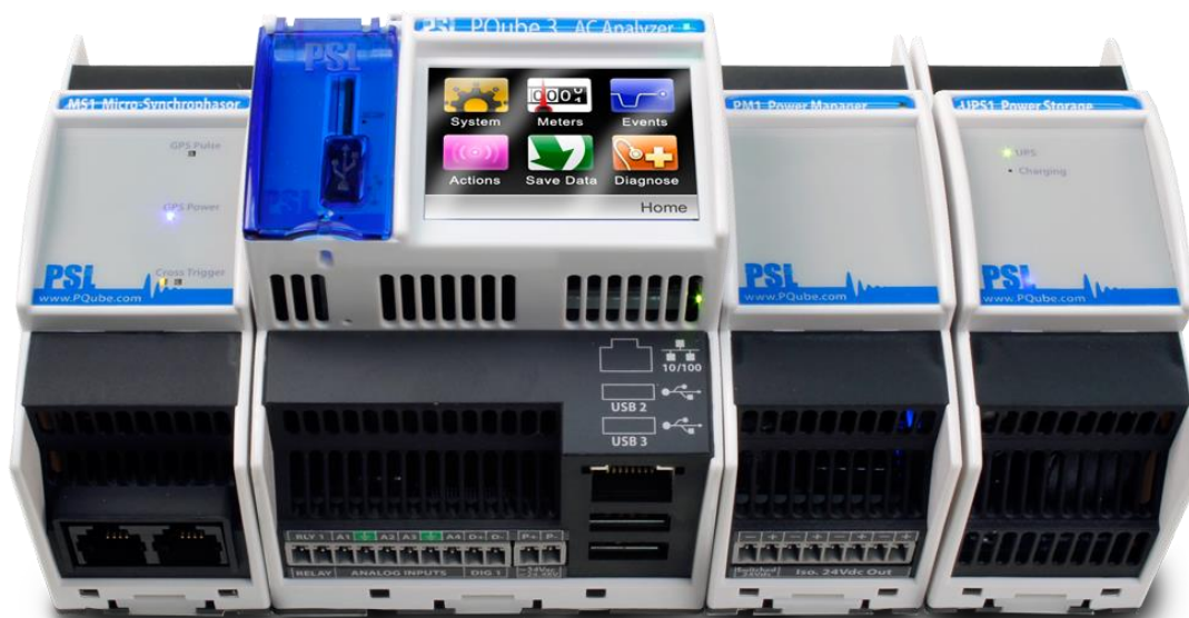
MS1 module on left side of PQube 3
