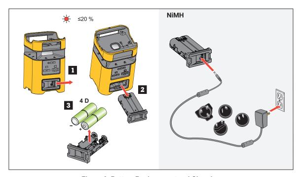
Figure 8. Battery Replacement and Charging
