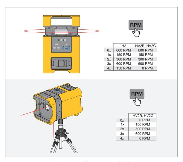
Figure 2. Revolutions Per Minute (RPM)
