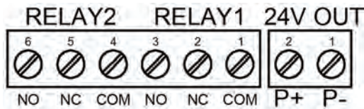
Figure 12. Relay & 24 V Output Connections
