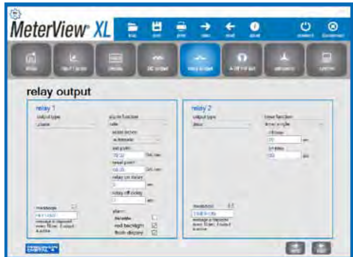
▲ The Relay Output window is used to assign a specific task to the 2 relays such as alarm, sample, timer, stopwatch, or off. A custom message that will flash every 10 seconds can also be added.
