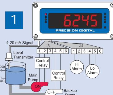
Relay #1 turns the main pump on at 6000 gallons and turns it off at 1000 gallons.
