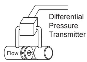
Display flow rate by extracting the square root of a signal from a DP transmitter.
