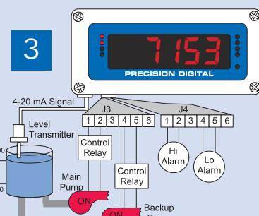
If backup pump is not able to keep up, and the level reaches 7000 gallons, relay #1 transfers and starts the main pump as well.
