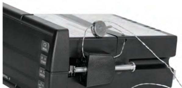
Figure 9: Close and Crimp Seal Wire Security Loop
