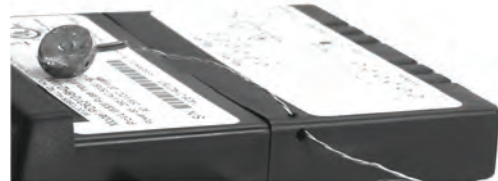
Figure 7: Wire Loop through Rear Case Pass-Through
