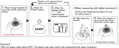
·When measuring hot samples, place only the necessary amount and do not let it overflow from the sample stage well. •When hot water is necessary to clean off hardened samples, use water-soaked gauze around the sample stage and keep hot water away from the body case.
