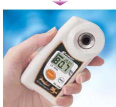
The Brix (%) will be displayed in 3 seconds. The PAL-LOOP will take continuous measurements, displaying the measured Brix value each second.
