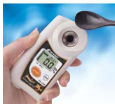
Apply 2-3 drops onto the prism surface.
